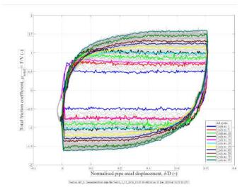
Total Friction Coefficient of the system increases with cyclic embedment.
