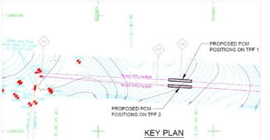
Pipeline Route showing Bathymetry and PCM location at Virtual Anchor Point.
