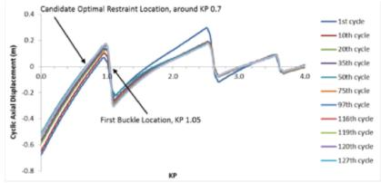
FEA Analysis used to identify Virtual Anchor Point.
